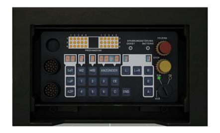
After entering the duration time and the mine density, it is determined from which side mines are fired. The launchers on both sides (key **L+R**), the left-sided launchers (key **L**) or the right-sided launchers (key **R**) can be selected.
