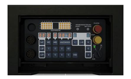
The "Einstell-, Prüf- und Abfeuergerät" (EPAG) is opened via the commander's mouse wheel menu. To start programming, the rotary switch (black, bottom right) is set to on (**EIN**) by clicking the right mouse button.
