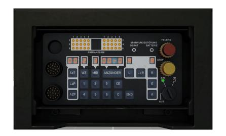
After entering the launcher side, the firing mode is finally set. To use the previously set parameters of the EPAG, the automatic mode is activated with the **A** key. Manual firing of mines can be set using the **E** key. After entering all parameters, the rotary switch is set to ready to fire (**FB**) by clicking the right mouse button again. The two firing modes **A** and **E** are explained on the following page (7+8).
