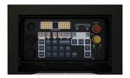
First, the duration time of the mine is set via the switch **WZ** followed by the entry of any number. The duration time is not simulated. Then the mine density is entered via the **MID** button. In automatic mode, this determines the distance between the individual bursts of fire.
